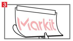
Peel the liner half-way and bend it back to meet the edge of the pre-mask. Keep exposed adhesive off surface.
