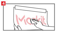
Allow vinyl decal to drape. Using firm initial squeegee pressure, continue at top center and work down and outward to each edge of mask.
